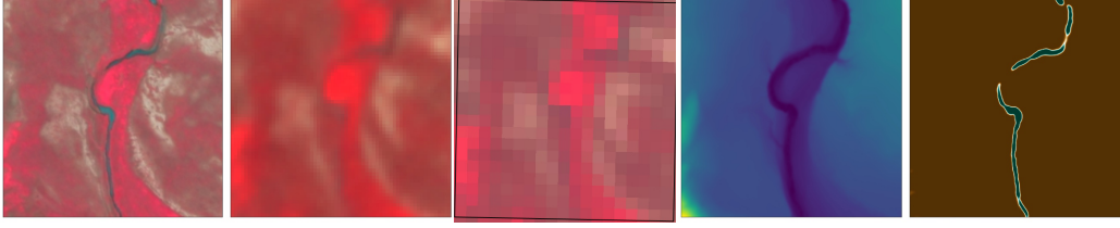
Figure 1: Narrow (5-2m) river in the South Dakota AoI. Left to right: WorldView 3 (WV3) (50cm/px), PlanetScope (3m/px), Sentinel-2 (30m/px), Digital Elevation Model (DEM) (1m/px), water probability map (50cm/px) of the same area. WV3, All satellite images are acquired on the same day, and are shown with a false RGB composite of Near-Infrared (NIR), Red, and Green bands.
