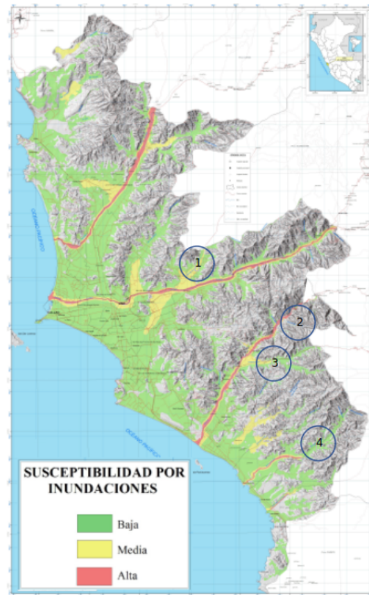
Figure 9: The flood susceptibility map provided by INGMMET. The blue circles indicate areas found by the algorithm with a high potential risk. Image from Villacorta Chambi et al. Peligros geológicos en el área de Lima Metropolitana y la región Callao N° 59 (Lima: Instituto Geológico, Minero y Metalúrgico, 2015)
